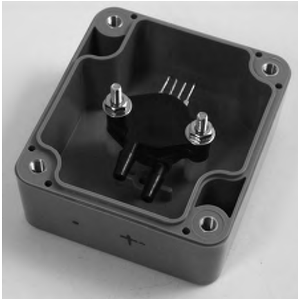
Figure 12-9. Transducer mounted inside weatherproof box using plastic spacers and M3 bolts
