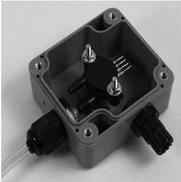
Figure 12-11. Transducer mounted with pressure hose fitted and cable gland for connection to Arduino in place
